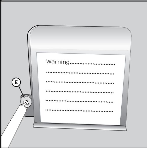
Replace junction box cover. Make sure the cover is seated behind the front lip of the strain relief plate. Attach the cover with the screw (part E) from the installation kit.
