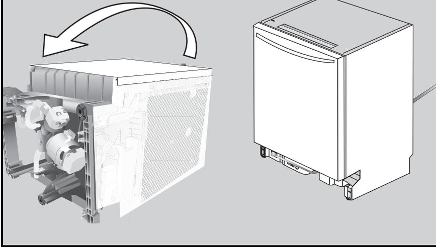
Flip unit back upright, ensuring water line is not pinched.
