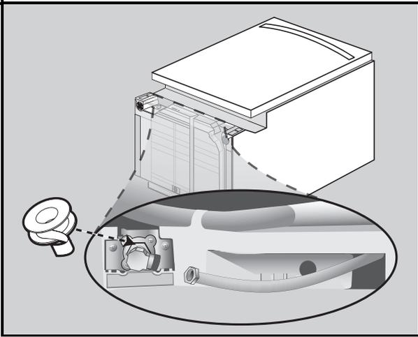
Attach 90° elbow joint to dishwasher oriented as shown, using thread seal tape when required. Do not over-tighten.
