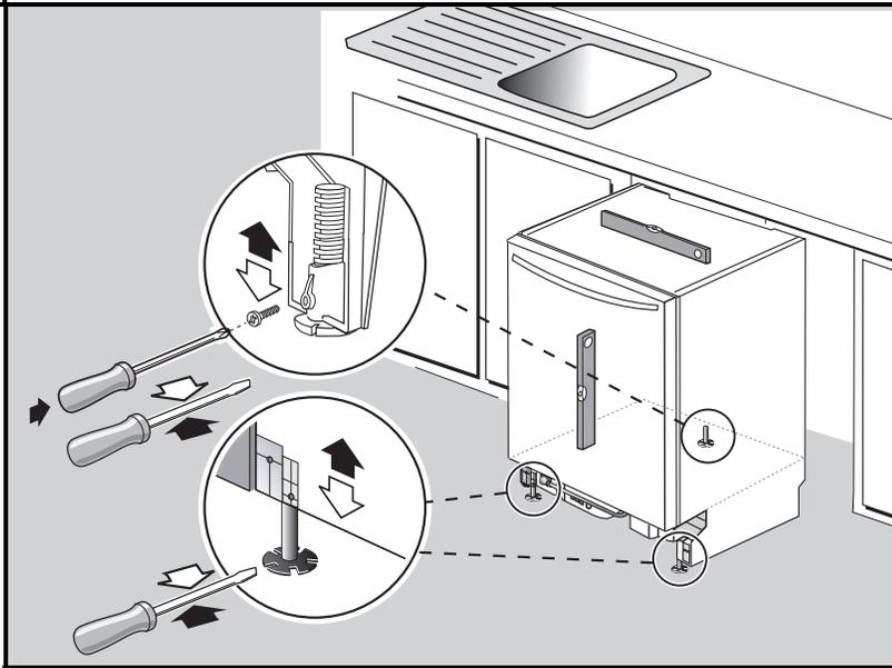
Pre-level unit before positioning under counter by turning feet clockwise to raise or counter-clockwise to lower. Maximum height the unit can be raised with feet fully extended is 34.5". Once the unit is at a satisfactory height, insert leg leveler locking screw (part F) in back foot. Step 18 will complete the leveling process.
