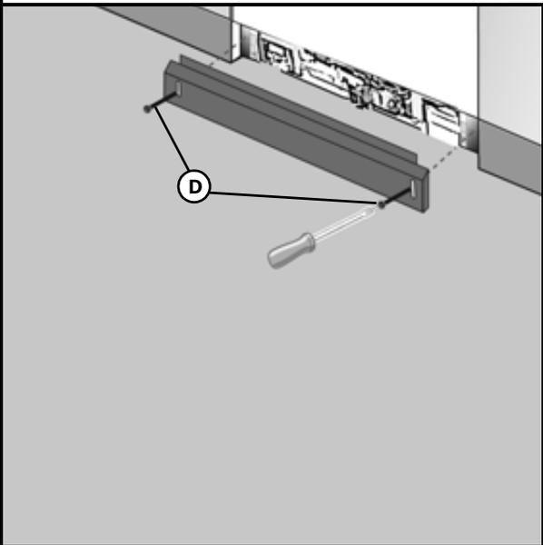
Attach the metal toe panel with screws (Part D) so it is flush with the floor. Success! Your installation is now complete.
