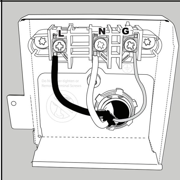
**Note: Do not loosen or remove terminal screws!** Damage may occur. Bend the wires so the exposed leads can reach the appropriate contacts. Insert the black (hot) wire into the left opening on the terminal strip marked "L", the white (neutral) wire in the middle opening of the terminal strip marked "N", and the bare copper or green (ground) wire into the right opening of the terminal strip marked "G". **Hand tighten only. Do not use power tools.**
