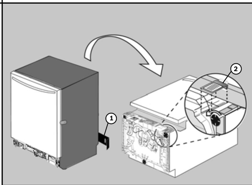
Remove the toe panel (1) from behind the unit and retain for attachment to the front at a later time. Loosen the leg levelers slightly. Remove junction box cover and retain for later use (2). Discard the small piece of protective styro-foam.
