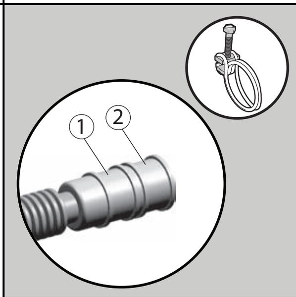
Attach drain hose to plumbing with screw clamp (position 1 for  $\frac{1}{2}$ " connection or position 2 for  $\frac{3}{4}$ " connection) and tighten. Do not cut drain hose.
