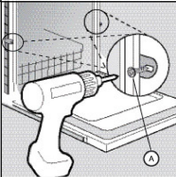
Insert screws (part A) through pre-positioned mounting brackets on each side of the unit and attach to enclosure (pre-drilling of holes recommended). Remove top rack before inserting screws.
