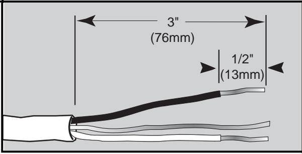
Strip outer casing of electrical wire to expose 3" (76 mm) of the inner wires. Then strip 1/2" (13 mm) casing from each individual wire.\*
