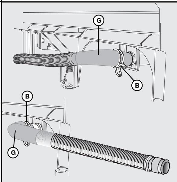
Orient hose toward direction of sink. **IMPORTANT:** Route hose toward sink PRIOR TO connection. Do not turn after attachment. Attach drain hose elbow (Part G) to back of unit using pliers to install the spring clamp (Part B).
