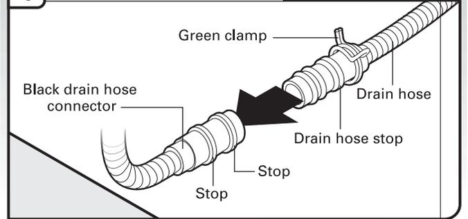
Place towel under drain hose to catch any water in drain hose. Place the small green drain hose clamp onto the small end of the drain hose. Push the new drain hose into the black drain hose connector up to the drain hose stop.
