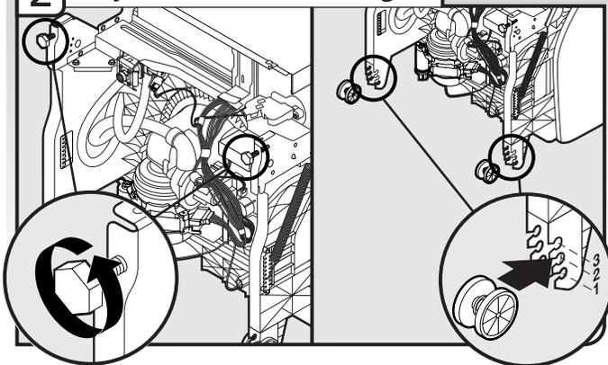
Turn both leveler legs to the same height. Put wheels in the required position determined from "Dishwasher Height Adjustment Chart." To change wheel position, use a flat-blade screwdriver to pop out the wheel, then snap into the new position.
