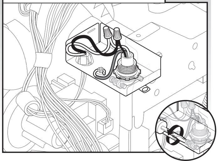
Tighten strain relief screws to secure cord.
