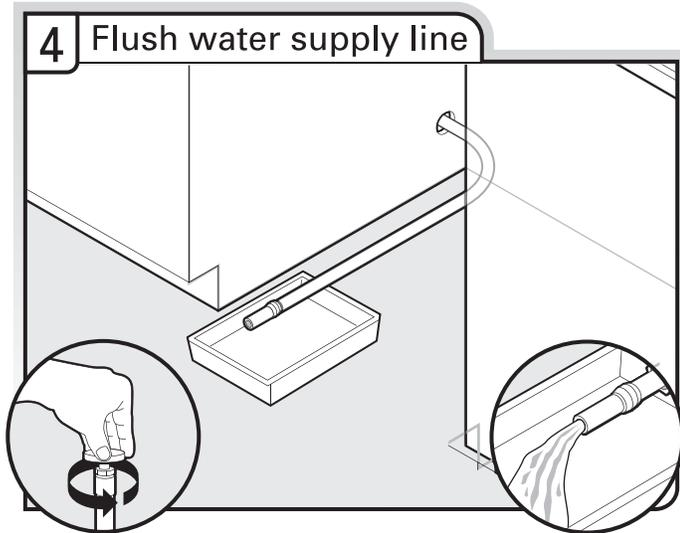
Slowly turn water shutoff valve to "ON" position. Flush water into a shallow pan until clear to get rid of particles that could clog the inlet valve. Turn shutoff valve to "OFF" position.
