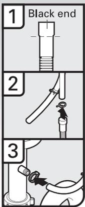
1. Connect black end of drain hose to air gap and cut if needed.
