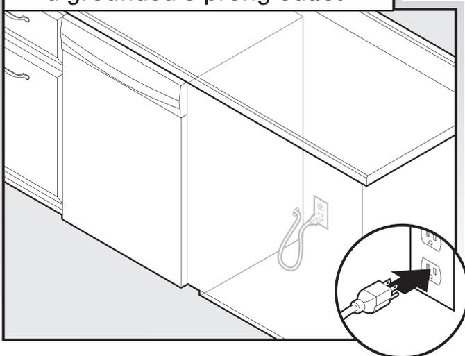
Plug into a grounded 3 prong outlet. Check that power supply cord does not touch dishwasher motor or lower part of dishwasher tub.
