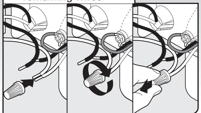
**NOTE:** Do not pre-twist stranded wire. Twist on UL listed/CSA approved wire connector. Gently tug on wires to be sure both are secured.
