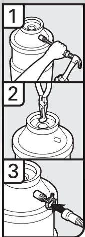
1. Using a hammer and screwdriver, knock plug into disposer.
