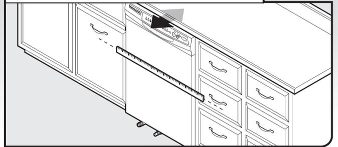
Align front of dishwasher door panel with front of cabinet doors. You may need to adjust alignment to be even with your cabinets.
