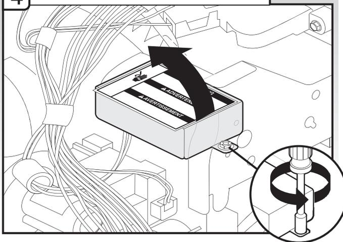
Using a  $\frac{1}{4}$ " hex head socket, nut driver or Phillips screwdriver, remove terminal box cover. Retain for later use.
