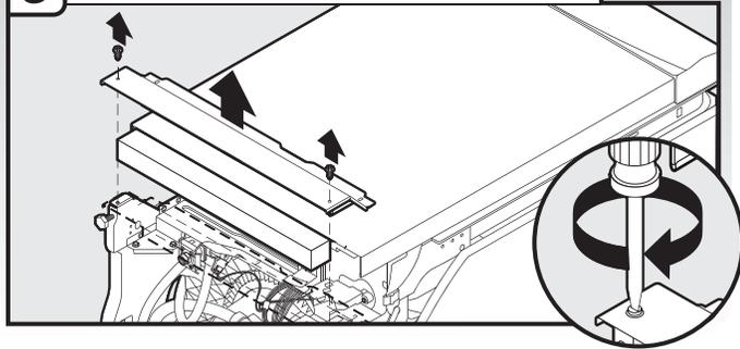
Using a flat-blade screwdriver, turn the plastic fasteners  $\frac{1}{4}$  turn to unlock them. Remove panel. Do not remove tech sheet from access panel.
