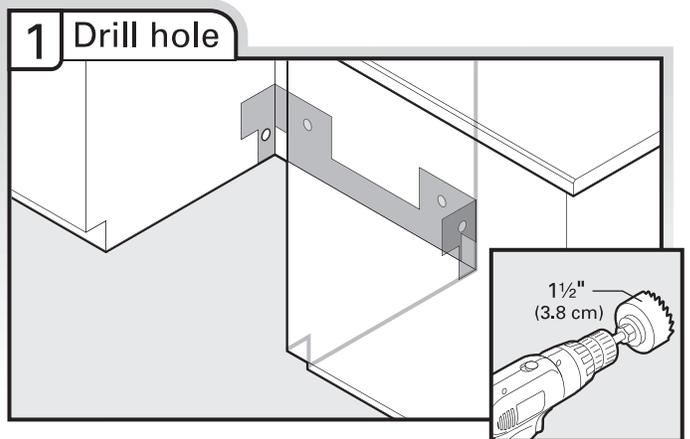
If needed, drill a 1½" (3.8 cm) diameter hole in cabinet wall or side of the opening closest to the sink.
