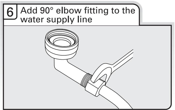
Connect the  $\frac{3}{8}$ " compression fitting to the water supply line prior to installing the unit into the cabinet opening. Attach such that the  $\frac{3}{4}$ " connection is facing upward as shown above.
