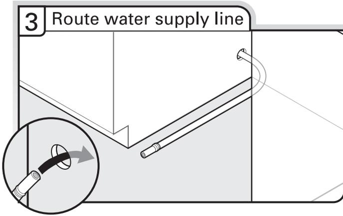
Slowly route water supply line through hole in cabinet. (If you are using copper tubing, it will bend and kink easily, so be gentle.) It should be far enough into the cabinet opening to connect it to the dishwasher inlet on the front left side of the dishwasher.
