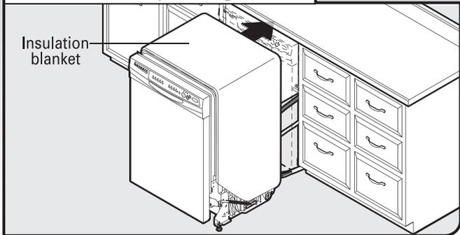
**IMPORTANT:** If wheels were removed, cover the floor when moving the dishwasher. Slowly move dishwasher completely into cabinet opening. Do not kink or pinch water line, drain hose, power supply cord or direct wire between dishwasher and cabinet. Remove cardboard from under dishwasher.
