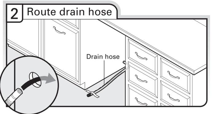
Route drain hose as shown through hole in cabinet to the front center of opening where drain connection will be made. Tape drain hose to the floor in area shown. This will prohibit it from moving when dishwasher is moved into cabinet opening.
