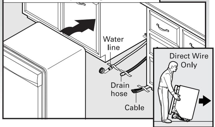
**IMPORTANT:** Double-check correct placement of utilities. Grasp the sides of the dishwasher at the edges of the door panel. Tilt dishwasher backward on wheels and move dishwasher close to cabinet opening.
