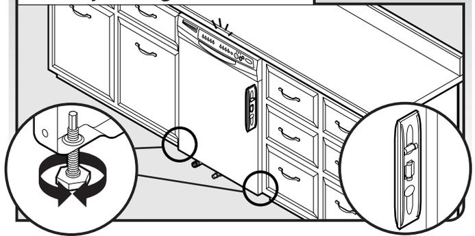
Check that leveling legs are firmly against the floor. Close and latch the door, and place level against the front panel. Check that dishwasher is centered from front to back in the opening. If needed, adjust leveling leg until dishwasher is plumb. Repeat for other side of dishwasher.
