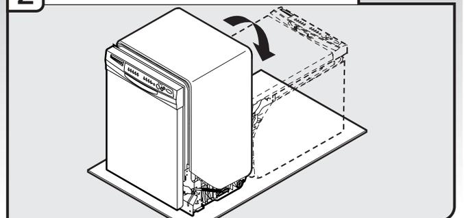
**Helpful Tip:** Place cardboard under dishwasher until installed in cabinet opening to avoid damaging floor covering. Do not use door panel as a worktable without first covering with a towel to avoid scratching the door panel.
