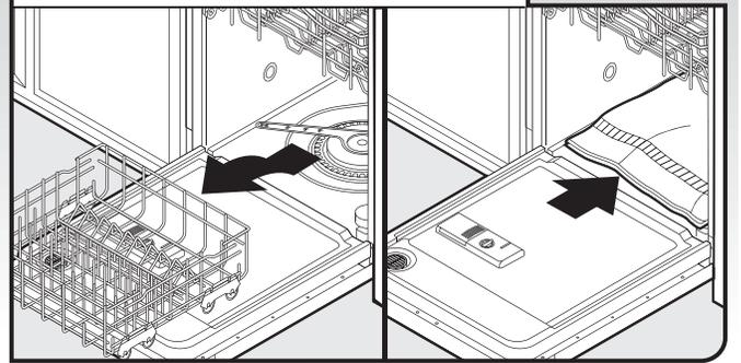
Open dishwasher door, remove lower dish rack, and place towel over pump assembly and lower spray arm of dishwasher. This will keep screws from falling into pump area when you are securing dishwasher to countertop.
