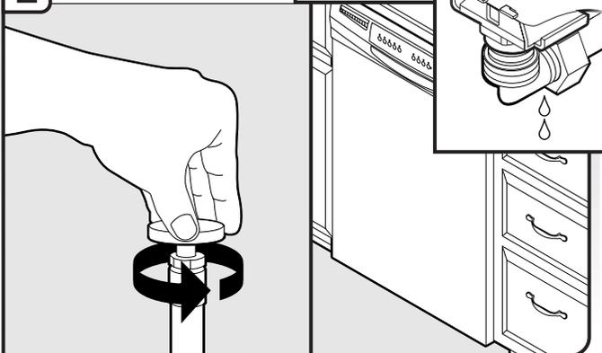
Place paper towel under 90° elbow fitting. Turn on water supply and check for leaks. If leak occurs, repeat previous step. If needed, see website for animated representation of this step. Visit [www.whirlpool.com/watersupply](http://www.whirlpool.com/watersupply) under FAQ tab.
