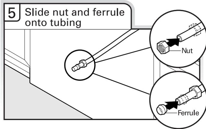
Copper tubing only: Slide nut, then ferrule, about 1" (2.5 cm) onto copper tubing.
