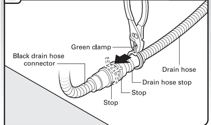
Using pliers, squeeze open the small green drain hose clamp and slide onto connector between stops.
