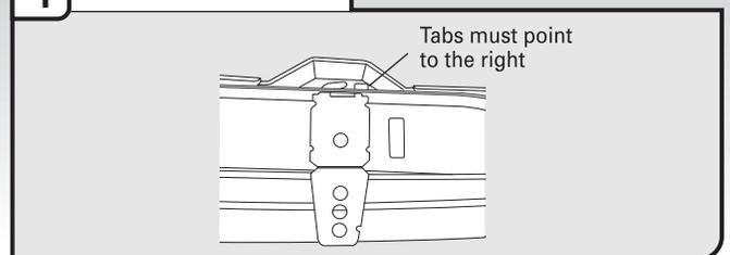
Remove the brackets from the package and insert into the open slots on the left and right-hand top of the dishwasher collar as shown.
