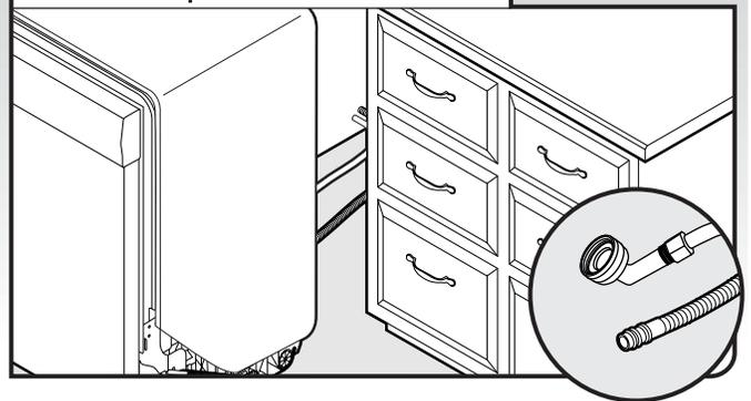
Check that water line is on the left side of opening and drain hose is near the center of the cabinet opening.
