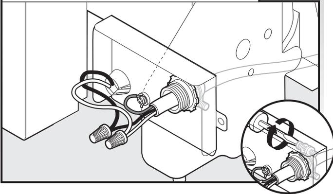
Tighten strain relief screws to secure cable.
