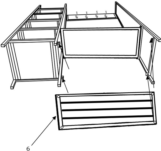
**STEP# 8:** Tighten the bolts to lock the iron shelf(6) as shown below.
