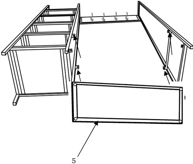
**STEP# 6:** Tighten the bolts to lock the wooden shelf(5) as shown below.
