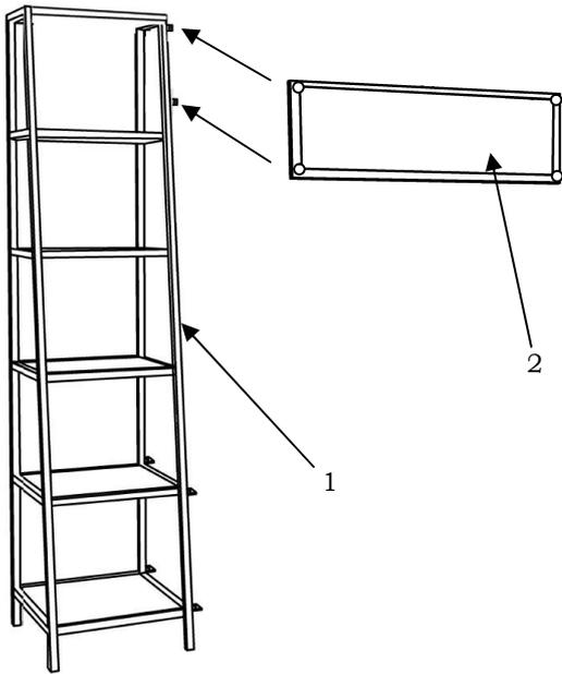
**STEP# 2:** Tighten the bolts to lock the hook board (2) as shown below.
