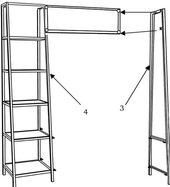
**STEP# 4:** Tighten the bolts to lock the iron stand(3) as shown below.
