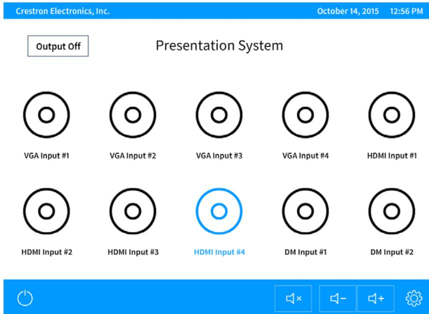
All enabled inputs are shown on this screen. Tap an input to route it to the output while the associated audio is routed to the analog audio output.
