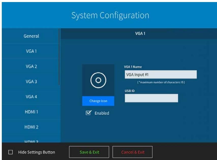
Use the **Name** text box to enter the input name you want to display on the source selection screen (shown on page 23).
