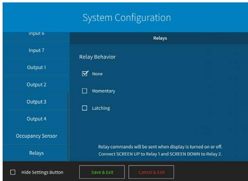
Relay commands are sent when the display is turned on or off. Connect SCREEN UP to Relay 1 and SCREEN DOWN to Relay 2.
