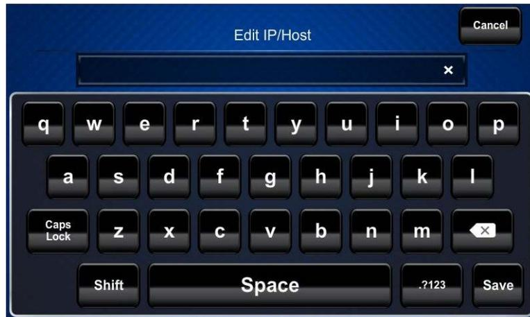
6. Enter the IP address or hostname of your host device using the on-screen keyboard. Tap **Save** to save the new entry and return to the **Ethernet Setup - Edit IP Table Entry** screen. Tap **Cancel** to return to the **Ethernet Setup - Edit IP Table Entry** screen.
