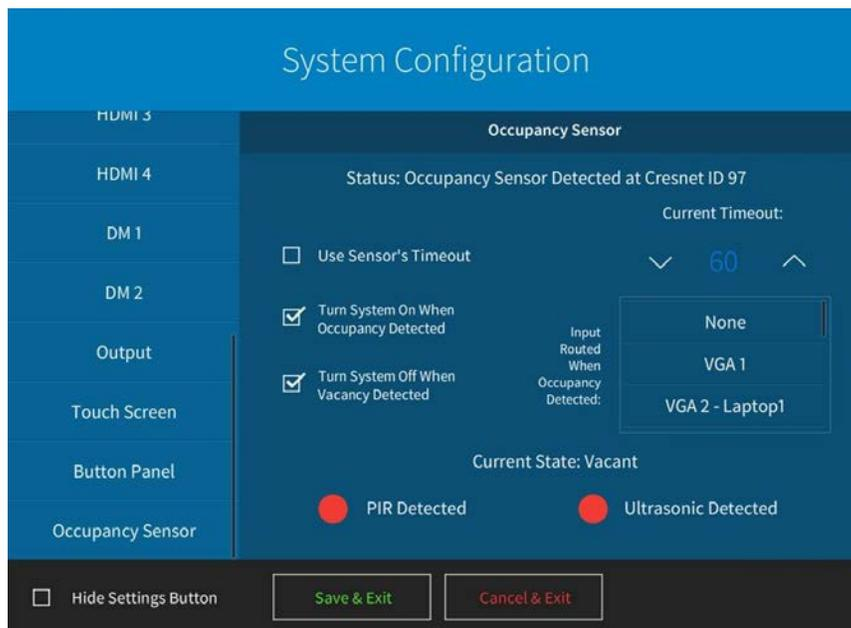
**NOTE:** The GLS-ODT-C-CN is detected at Cresnet® network ID 97.
