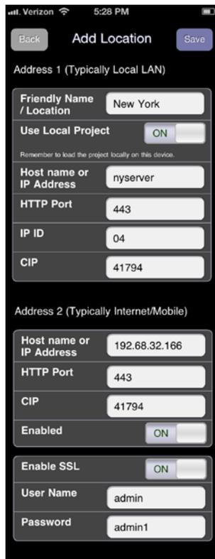
3. In the **Address 1 (Typically Local LAN)** section, enter the configuration information for a Wi-Fi® connection.
