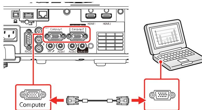
4. Tighten the screws on the VGA connector.
