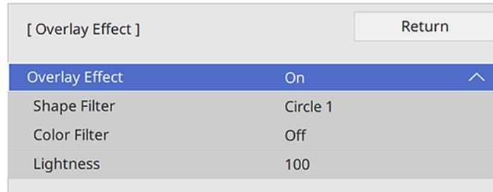
3. Select the **Shape Filter** setting and adjust the options as necessary.
