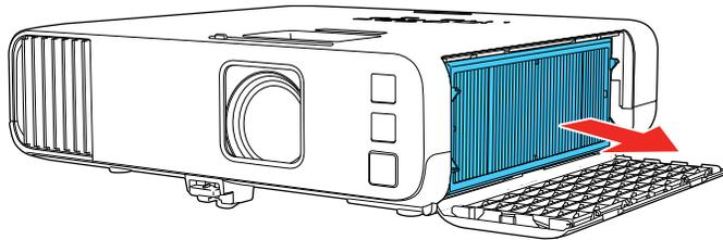
**Note:** Air filters contain polypropylene. Dispose of used air filters according to local regulations.
