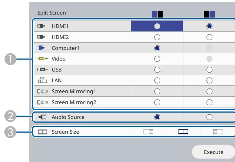
4. Press the arrow and **↵ Enter** buttons to select an image source for each section of the screen.
