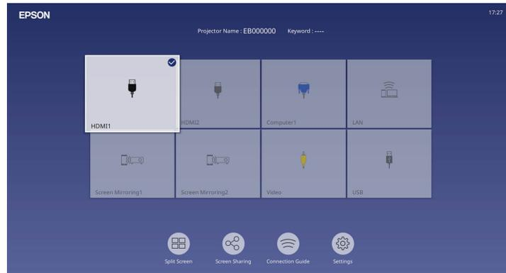
**Note:** Your Home screen may look different from the illustration shown here. A checkmark appears on the image from the current input source. You can see thumbnail previews of most input sources (except the USB input source when in Content Playback mode [EB-L260F/EB-L265F]).
