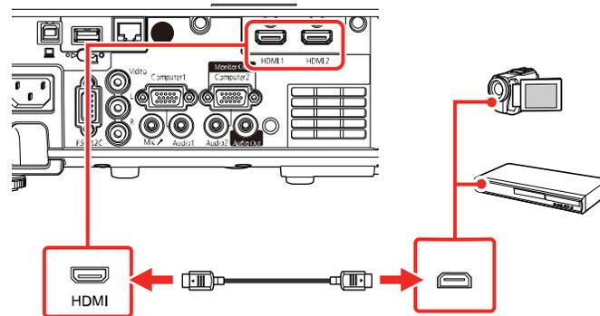
**Note:** The projector converts the digital audio signal sent from your video source into a mono analog signal for the internal speaker or a stereo analog signal if you are connecting to external speakers.
