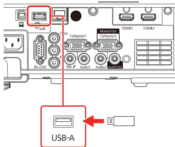
**Note:** Connect the flash drive directly to the projector. Do not use a hub or your settings may not be saved correctly.
