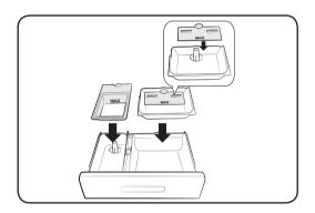
**3.** Remove the inserts from the 3 compartments. Rinse the inserts and the drawer with warm water to remove traces of accumulated laundry products.
