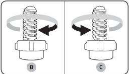
**3.** If the washer is level, the **pulsator** (A) will be positioned at the center of the tub as shown in the figure on the previous page. If it isn't, level your washer by turning the front leveling feet clockwise or counterclockwise as necessary.
