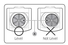
See if the washer is level by checking the position of the tub:
