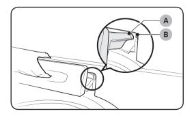
5. Return the inserts to their proper compartments, and then replace the drawer by placing the dispenser drawer rail (B) on top of the compartment rail (A) (To make this easier, tilt the dispenser drawer downward and insert it). Then push the drawer in firmly and slowly.
