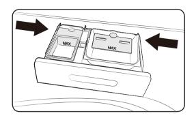
**2.** Push in both sides of the drawer at the back simultaneously. When you feel the sides move inward, pull out the dispenser drawer.
