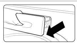
The automatic dispenser may need to be cleaned periodically due to laundry additive buildup.
