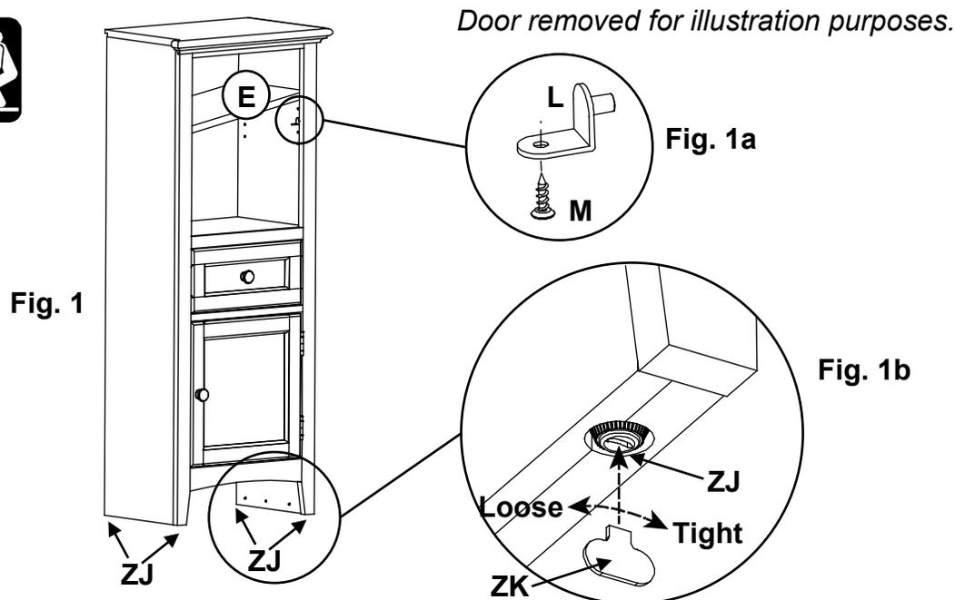
2. Place the unit at its final destination. Use the Leveler Adjustment Key (ZK), found in the Zip bag taped to the Owner's Manual and Safety Guide to rotate the Slotted Levelers (ZJ) on the bottoms of the legs until the unit is level. See Figures 1 and 1b.
