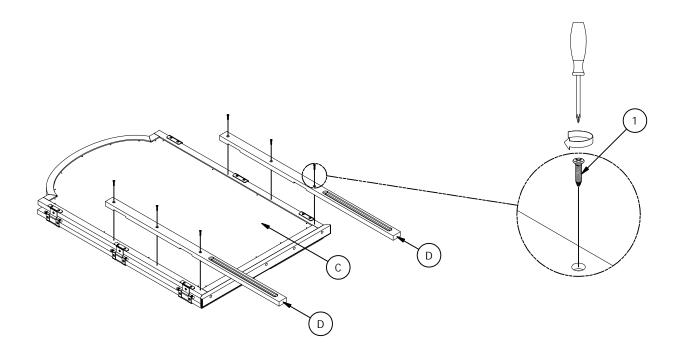
Step 2: Place all parts down on a piece of cloth or carpet to prevent finish from scratching. Insert the screw (1) in to the hole on the connecting bar (D) and then assemble with mirror (C), tighten with screwdriver (not provided).
