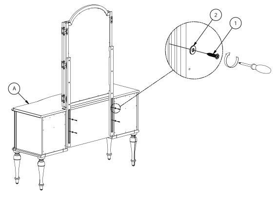
Step 3: Attach connecting bar (D) to vanity desk (A). Insert the screw (1), flat washer (2) into the groove on the connecting bar (D), tighten with screwdriver (not provided). Assembly product is now completed.
