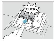
The detergent dispenser will open automatically at the ideal time for the set cycle. The powder or liquid detergent is distributed in the appliance and is dissolved, detergent tabs will fall into the detergent tab tray [22] where it dissolves during the cycle.
