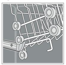
Re-insert the rack with the other set of roller guides as shown below.
