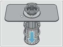
Rinse the filters under running water and use a soft brush to clean.
