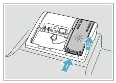
Add liquid rinse aid to the dispenser 28 until it is full. Do not overfill. Avoid spilling into air vent hole.
