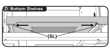
Push a shelf [07] onto the tabs (T) at the back of the rails. Lower the shelf [07] onto the rails. Push the shelf locks (SL) inward to secure the shelf. The shelf locks (SL) will click when locked into position.
