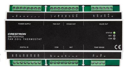
**DIGITAL IN:** (8) Captive screw terminals; Comprises (4) potential-free binary inputs
