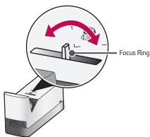
To bring images into focus, move the Focus Ring slowly left or right, concentrating on the upper central part of the screen. Optimal focus is reached when the left and right sides of the screen appear balanced.
