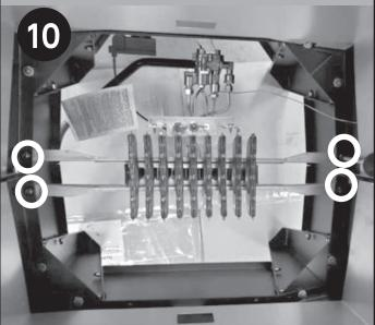
Remove the four (4) Screws holding the bracket.
