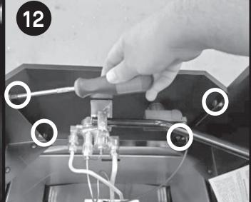
Remove four (4) Screws from control panel and remove the component.
