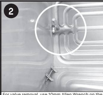
For valve removal, use 10mm Allen Wrench on the inside of the pot.
