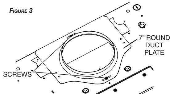
**NOTE:** To accommodate off-center ductwork, the 7" round duct plate can be installed up to 1/2" on either side of the hood center.
