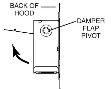
**TIP:** Insert a small length of duct over the 3 1/4" x 14" damper assembly and seal the joint using aluminum foil duct tape to ease connection with the house ductwork.
