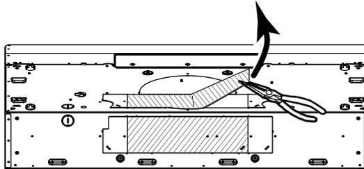
**9 ]** Attach 3/4" x 10" Damper Assembly on top OR back of hood (if using 3/4" x 10" duct; shaded part in **FIGURE 2 A** below) or 7" Round Duct Plate (if using 7-inch round duct, **FIGURE 3**) over the knockout opening. When installed, the 3/4" x 10" damper assembly must open as shown in **FIGURE 2 B**.
