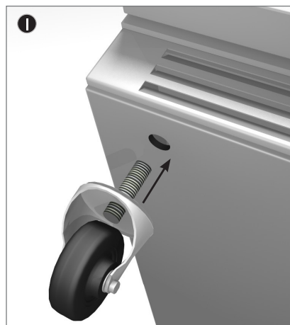
Thread castor into the underside of cabinet frame rail.
