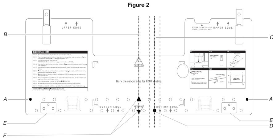
**NOTE:** If wall studs is within 6" (15.2 cm) of the vertical centerline (see "Mark Rear Wall" section), only recirculation or roof venting installation can be done.
