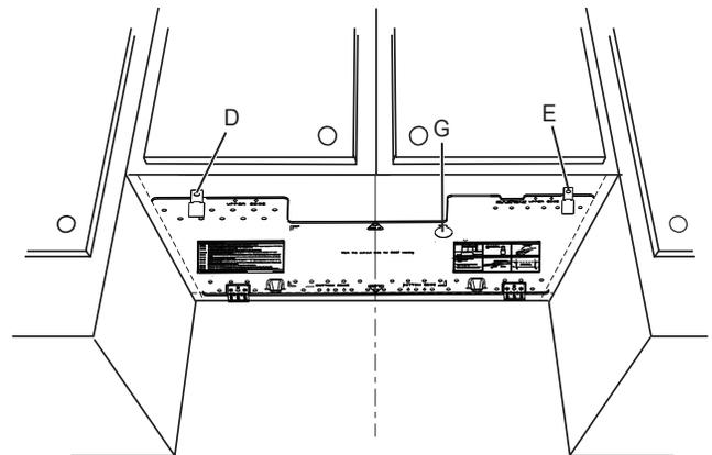
**Note:** If upper cabinet is metal, the supply cord bushing needs to be installed around the supply cord hole as shown.
