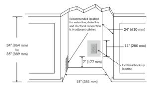
NOTE: For Gravity drain models, the drain hole cannot exceed 7 inches above the floor. models, the drain hole should be no lower than 7 inches and no higher than 4 feet above the floor.
