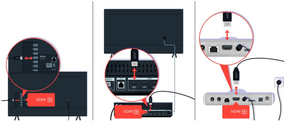
Check the antenna and HDMI cable connections.
