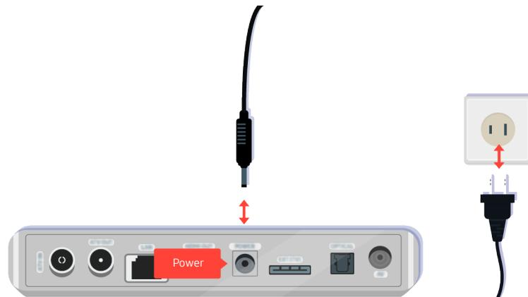
If it does not turn on, make sure the power cable is properly connected to the device and to the wall outlet.
