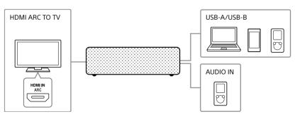
\* ARC is a feature to send TV sound from the HDMI input port of a TV to an AV device using the HDMI cable.
