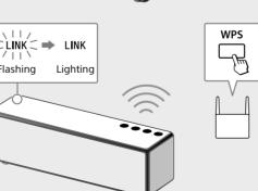
Depending on the wireless router, press and hold the Wi-Fi Protected Setup (WPS) button for a few seconds. For details, refer to the operating instructions of your router. When the LINK indicator lights up in orange, the Wi-Fi network connection is complete.
