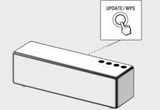
3 Within 90 seconds, press the Wi-Fi Protected Setup™ (WPS) button of the
