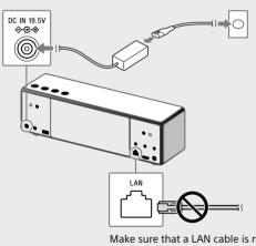
Make sure that a LAN cable is not connected. A wired and wireless connection cannot be used at the same time.
