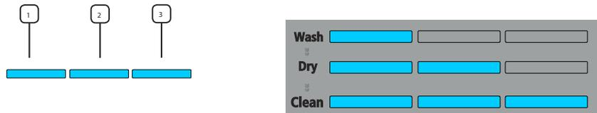
Located on the right side of the front of the dishwasher, these lights indicate the process in this running cycle.
