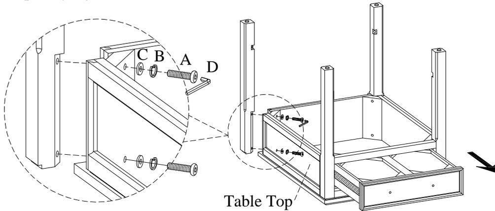
**STEP 2:** Attach the bottom shelf to legs by using 4 bolts(A), lock washers(B) and flat washers(C). Use the Allen wrench provided to tighten all the bolts. Push back the drawer. Turn the assembled table to the upright position.
