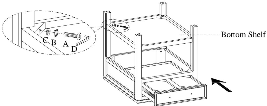
**STEP 3:** Reverse the handle by removing the screws while this drawer is open and attach the handle to the front of the drawer with screws as shown below.
