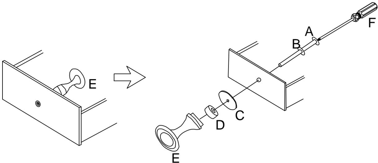
Place the accessories in the order shown above. Use a screwdriver to secure the handle to the outside of the drawer.
