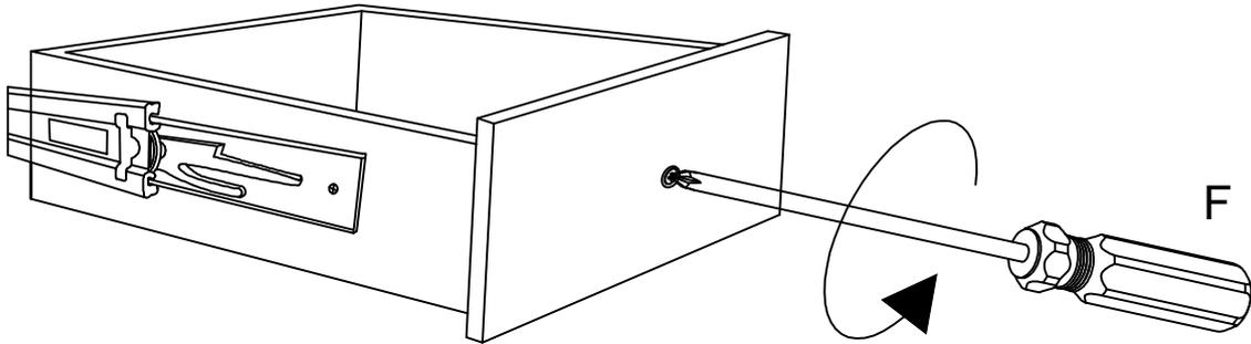
Open the drawer and remove the handle and accessories with a screwdriver.
