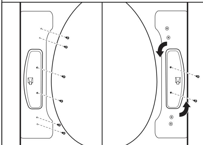
Using a T25® screwdriver, remove the two screws securing the door strike to the door frame of the dryer. Remove the four screws above and below the door strike and set aside for later use. Rotate the strike 180° and attach to the opposite side of dryer door frame, as shown.
