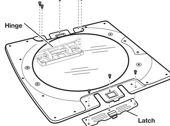
Using a T25® screwdriver, remove the three screws securing the latch plate and the five screws holding the hinge assembly in place.
