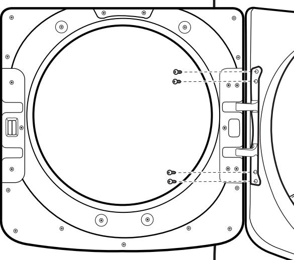
Using a T25® screwdriver, reinstall the four screws securing the door hinge to the dryer.
