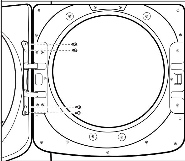
Using a T25®<sup>†</sup> screwdriver, remove the four screws securing the door hinge to the dryer and lift up and out to remove the door. Place the door on a soft towel or other non-scratch surface. Retain or set aside the four screws.
