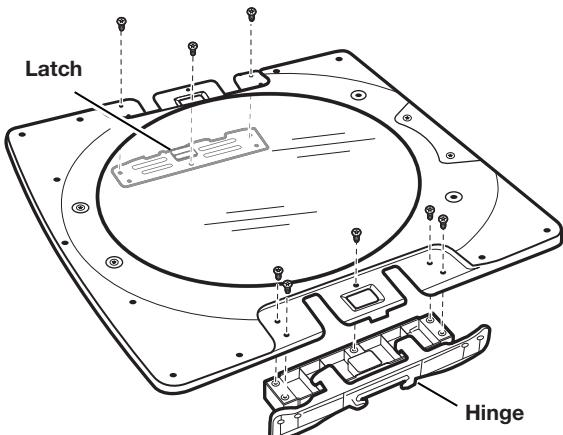
Using a T25® screwdriver, reinstall the latch plate and hinge assembly on the opposite sides from which they were removed.
