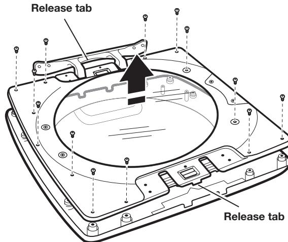
Position the door with the inside of the door facing up. Using a Phillips screwdriver, remove the 13 screws securing the inner door to the outer door. Lift off the inner door and set aside.
