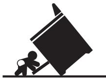
**▲ WARNING** If your range is removed for cleaning, servicing or any reason, be sure the anti-tip device is reengaged properly when the range is replaced. Failure to take this precaution could result in tipping of the range and can result in death or serious burns to children or adults.
