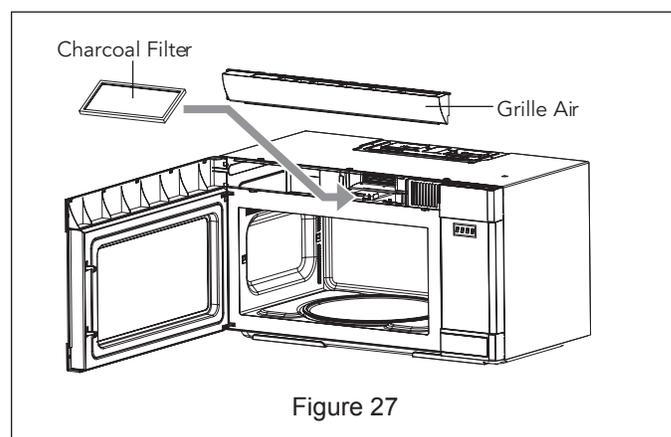
6. Replace the grille air and 3 screws and close the door.
