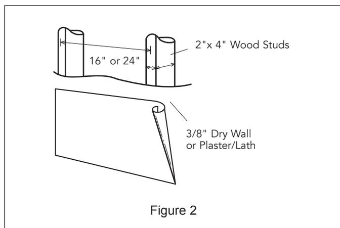
**NOTE:** In the event that the unit will be unable to be supported by any stud, it will be necessary to use special care in the placement of the toggle bolts and top cabinet screws. See Wall Template for details. The top cabinet should be tested to ensure it is securely attached to the wall. Place extra weight up to 110 pounds inside the top cabinet to test the support.
