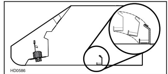
It is recommended to install side filters first and finish with middle one(s).
