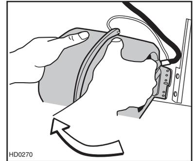
Flip the blower and engage its flange in the back wall retaining bracket.
