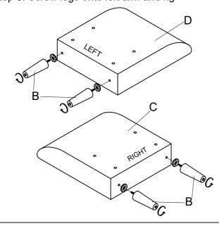
Step 4: Screw leg onto the bottom frame
