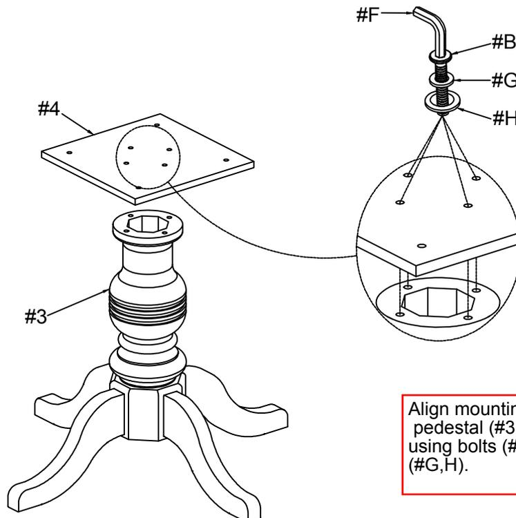
Align mounting plate (#4) to the pedestal (#3), then secure by using bolts (#B) with washers (#G,H).
