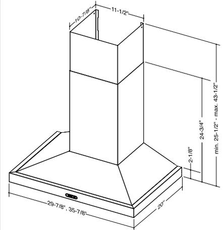
Install hood so that the bottom of the unit is 24" to 30" above the cooking surface. Mounting height may be affected by ceiling height.
