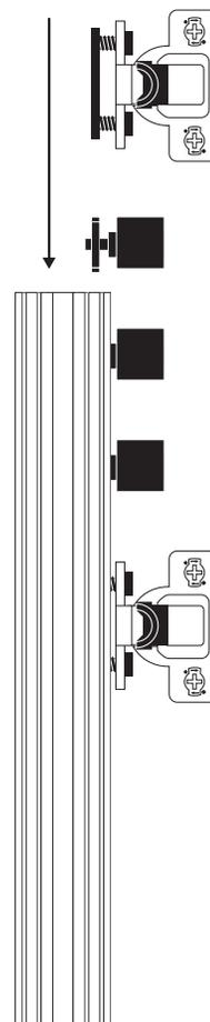
1. Slide the bottom hinge plate through front post channel.
