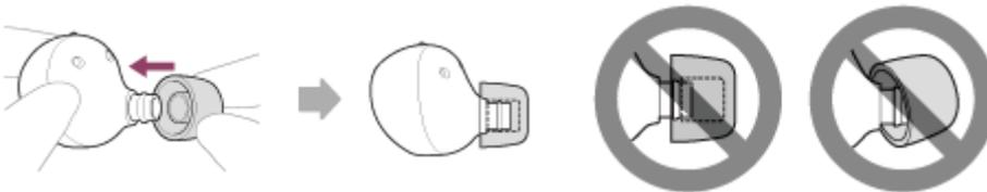
If the earbud tip is not completely attached, the earbud tip may be removed from the headset and the sound quality, noise canceling effects, and wearability may be impaired.
