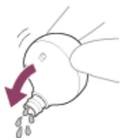
3. Turn the microphone part or air hole part downward and gently tap it about 20 times on a dry cloth, etc. to remove any water collected inside.
