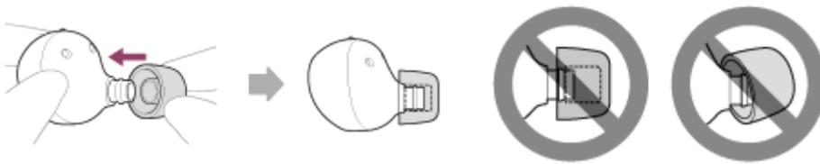
If the earbud tip is not completely attached, the earbud tip may be removed from the headset and the sound quality, noise canceling effects, and wearability may be impaired.
