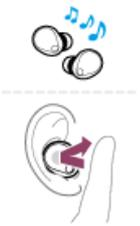
Tap the center of the touch sensor with the pad of your index finger.
