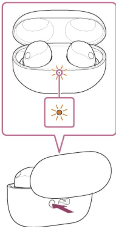
Then, the indicator on the charging case turns off and the headset will be reset.
