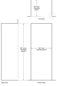
NOTE:  $3^{1/2^{*}}$  (89) finished returns will be visible and should be finished to match cabinetry.
