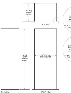
NOTE: 3<sup>1</sup>/2" (89) finished returns will be visible and should be finished to match cabinetry Shaded line represents profile of unit.
