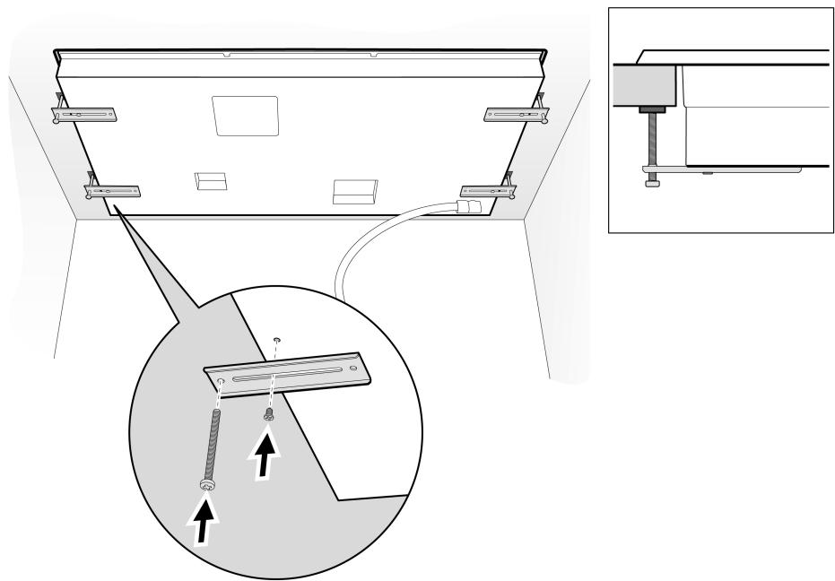
The cooktop should be secured to the countertop using the clamping brackets provided.
