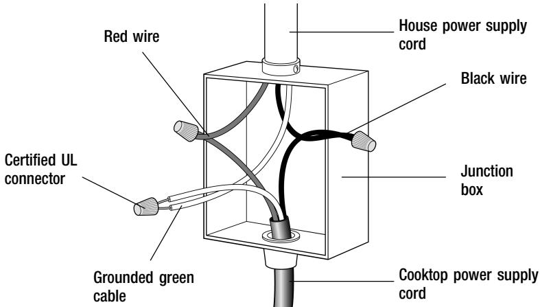
If the cooktop is installed and connected as specified above, it will be completely grounded in compliance with the National Electrical Code.
