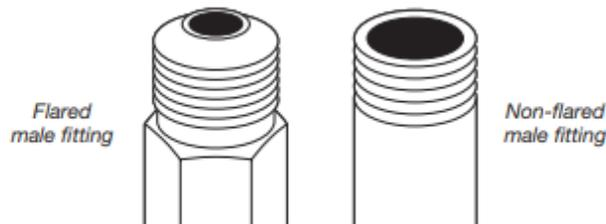
Remove red cap from gas pipe. Using a wrench to tighten, connect gas supply to dryer. Use pipe-joint compound on threads of all non-flared male fittings. If flexible metal tubing is used, be sure there are no kinks.
