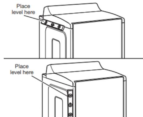
Check levelness of dryer from side to side. Repeat from front to back.
