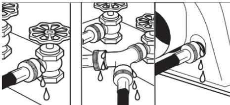
Check for leaks around "Y" connector, faucets, and hoses.
