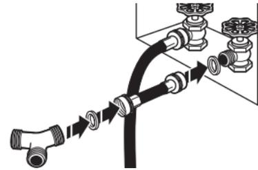
Attach 2 ft (0.6 m) inlet hose to cold water faucet. Screw on coupling by hand until it is seated on faucet. Then attach "Y" connector to male end of the 2 ft (0.6 m) inlet hose. Screw on coupling by hand until it is seated on connector.
