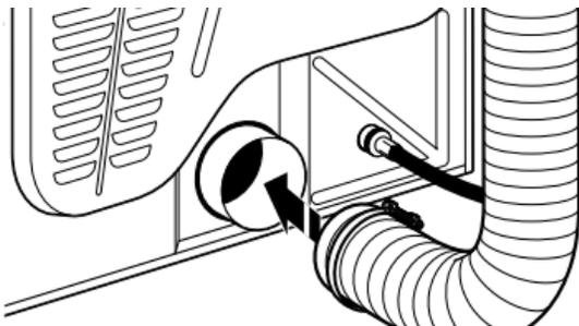
Using a 4" (102 mm) clamp, connect the vent to exhaust outlet in the dryer. If connecting to existing vent, make sure vent is clean. Dryer vent must fit over dryer exhaust outlet and inside exhaust hood. Check that vent is secured to exhaust hood with a 4" (102 mm) clamp.
