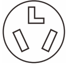
3-wire receptacle (10-30R)
