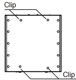
Place charcoal filters to back side of baffle filters. Secure charcoal filters in place by rubber clips. Depending on filter design secure top and bottom of charcoal filters by either rubber clips.
