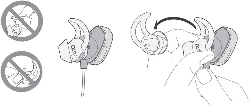
2. Align the opening of the new StayHear<sup>®</sup>+ Pulse tip with the earbud nozzle and rotate the tip onto the nozzle.
