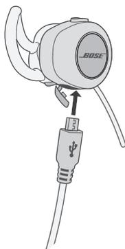
3. Plug the other end into a USB wall charger or computer that is powered on.
