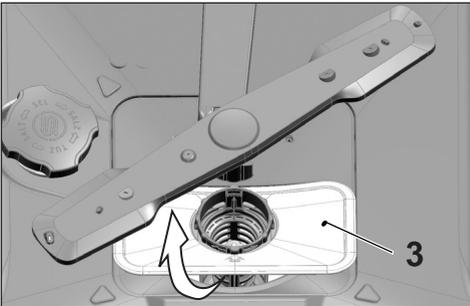
3. Press the two pawls on the coarse filter inwards and separate the coarse filter from the assembly.
