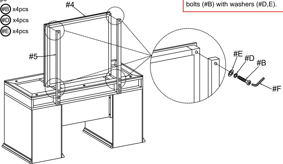
Align mirror (#4) to the mirror supports (#5), then secure by using bolts (#B) with washers (#D,E).
