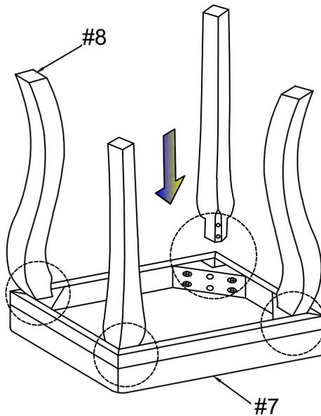
Align legs (#8) to the seat (#7), then secure by using bolts (#C) with washers (#D,E).
