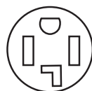
4-wire receptacle (14-30R)
