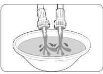
3. Put the other ends of the hoses into a bucket, and then open the water taps for 10 - 15 seconds to remove impurities. When done, close the taps.
