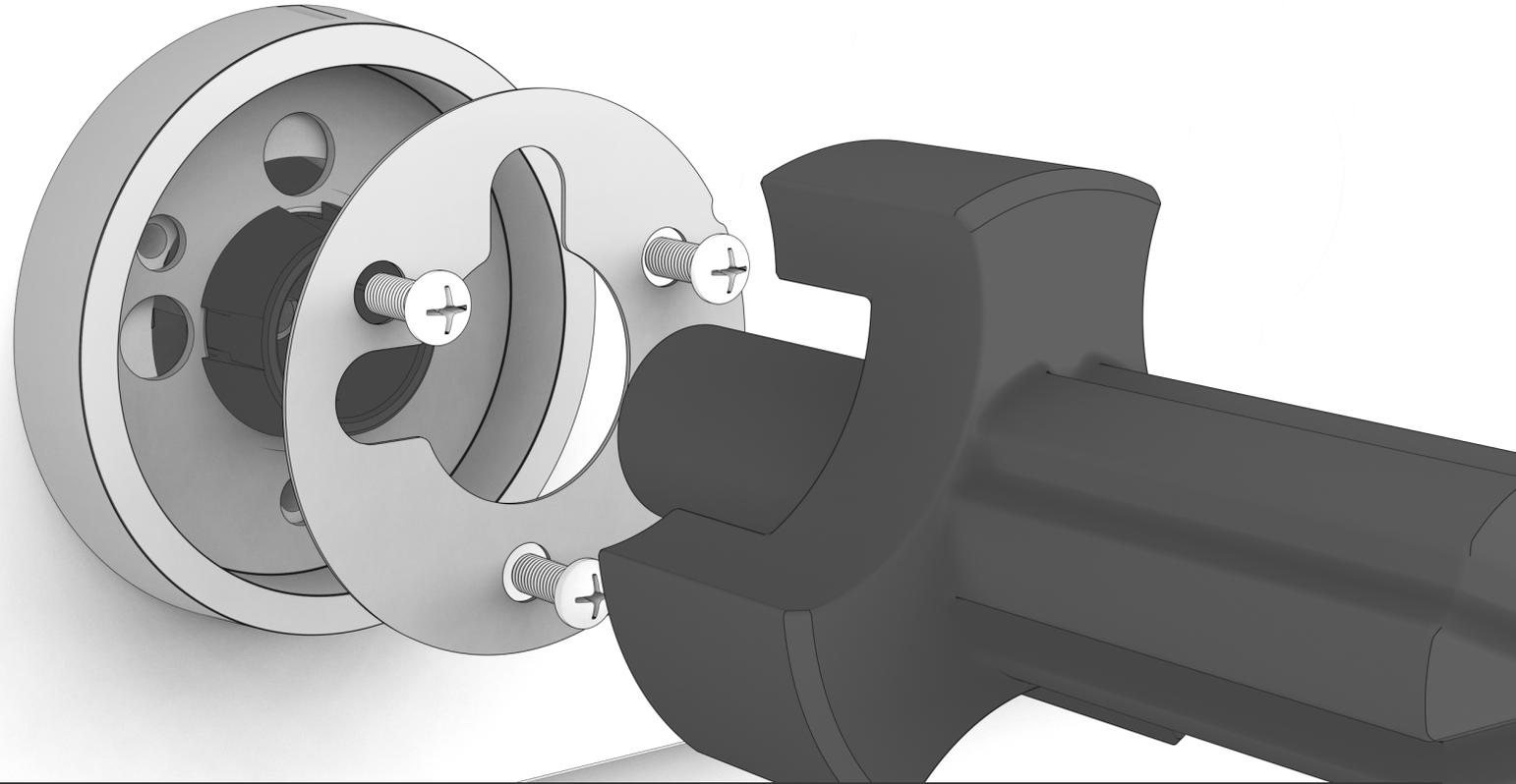
**IF THE FLANGE IS PRESENT, REPOSITION IT IN THE CORRECT POSITION**
