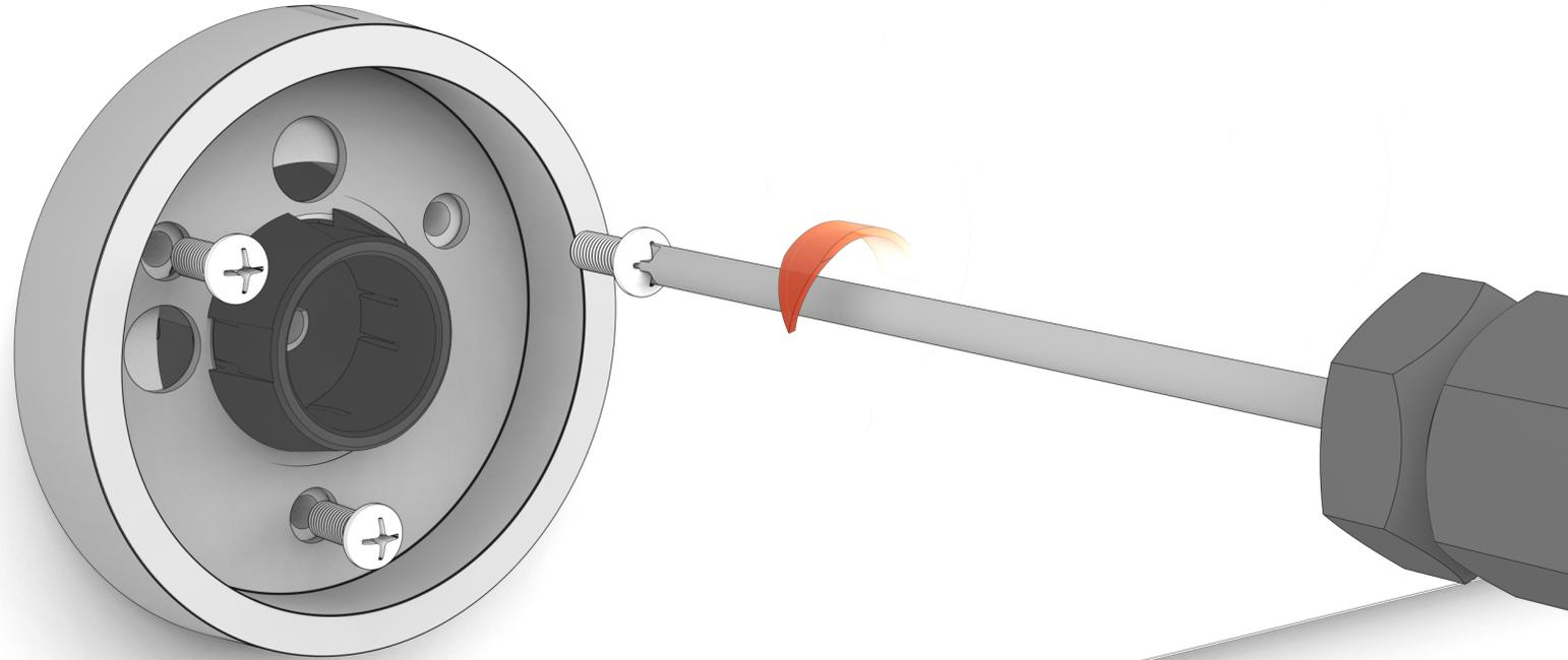
HOLD BEZEL WHEN REMOVING FINAL SCREW
