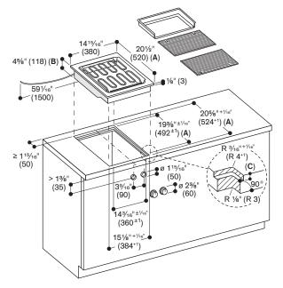
Minimum countertop thickness  $1^{3}/\omega''$  (30 mm) for flush installation. See separate planning notes on page 106.
