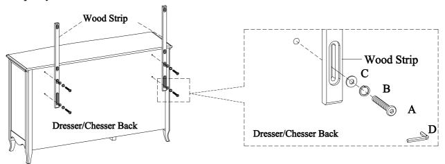
STEP 2: Attach the wood strips to the mirror by using 4 bolts(A), lock washers(B), and flat washers(C). Tighten all bolts on dresser and mirror with Allen wrench.
