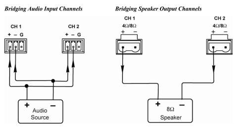
**NOTE:** The **INPUT LEVEL** controls for both channels must be set to the same level.
