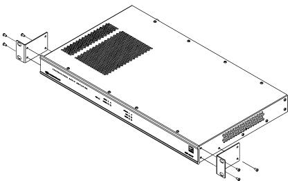
4. Repeat procedure (steps 1 through 3) to attach the remaining ear to the opposite side.
