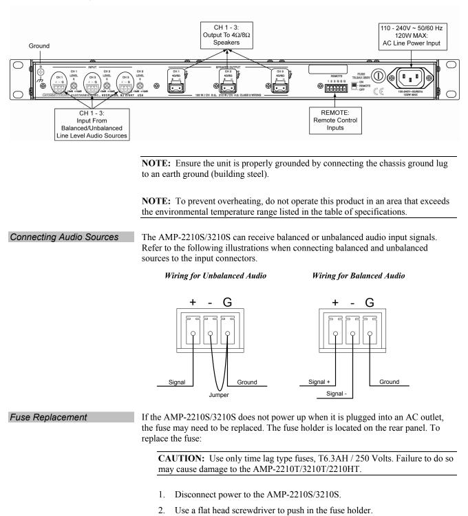
3. While pushing in the fuse holder, turn screwdriver counterclockwise until the fuse holder pops out.
