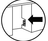
IN TIGHT INSTALLATIONS **CUT THROUGH AN ADJACENT** CABINET WALL TO REACH AN OUTLET INSTALLED THERE
