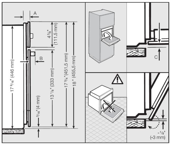
A 7/8" (Appliance with glass front: 22 mm / Appliance with metal front: 23 mm)
