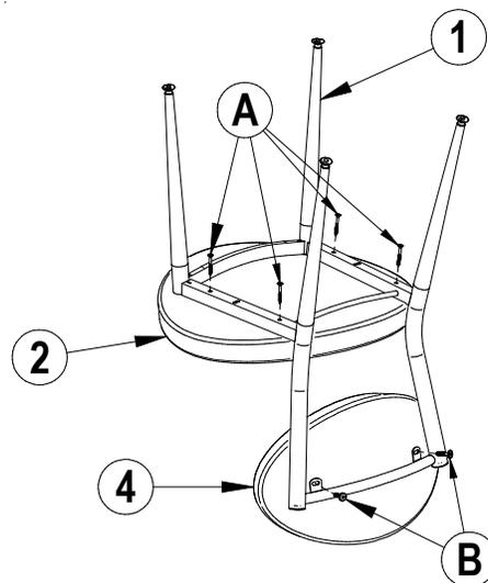
3) Screw-on the upholstered backrest (front part) **4** on the upholstered backrest (rear part) **3** with bolts **B**.
