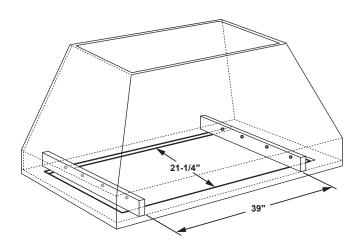
These hoods are secured to the custom cabinet from both sides through 8 screws.
